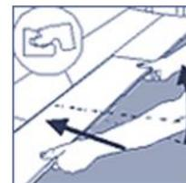
14. Tip: This movement requires some gentle adjustments on the pressing angle. Adjust the distance to the wall to 10 mm when three rows are completed.
