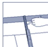
18. The last and first plank can be cut in the correct width. Place the last plank on top the second to last plank.
