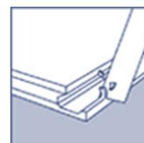
23. Glue (PVA Glue, class D3). Install the plank
