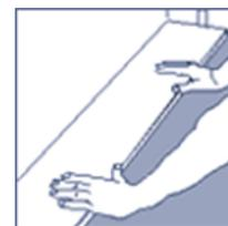
6. Hold the next plank against the first at an angle to the first one and lay it flat on the floor.
