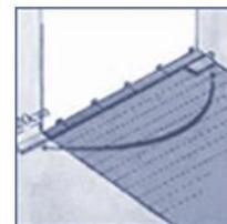
8. If you are installing floating floor planks, start the next row with the piece left, must be at least 300 mm long). Always ensure that the end joints are staggered at least 300 mm. CorkComfort Floating, tiles 605 x 445 "brick" or "half brick" installation method must be used. Place the final plank face down and the short side without the locking strip towards the wall. The distance to the wall should be 10 mm.
