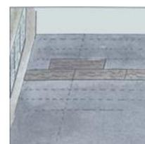
4. If you are installing Wood floors with three strips, try not to match the strips of the tiles.
