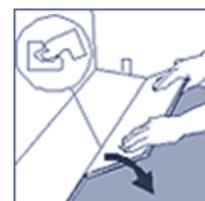
12. Place the short end of the plank at an angle against the previous installed plank and fold down.
